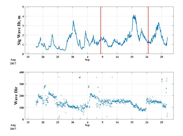
Figure 3. Recent significant wave height and direction data from the NDBO buoy 44025 located some 30 nautical miles south of Long Island. The red lines indicate the times of photo flights over the breach shown in Figures 1b and 4.
