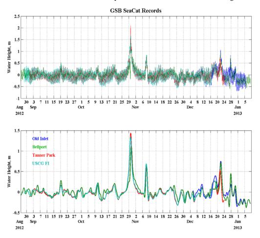
Figure 2. Water level records from the Old Inlet area, Bellport, Fire Island USCG base and Tanner Park. The lower panel shows the low-passed height records using a 33 hour half-power symmetric filter.
