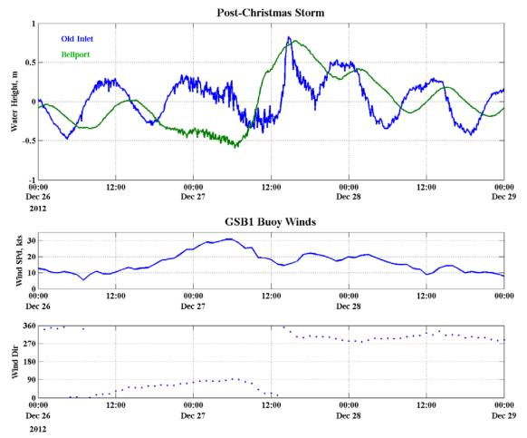
Figure 7. Water levels and Bellport and Old Inlet, and winds from the GSB1 buoy during the December 27th storm
