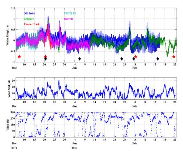
Figure 2, Time series plots of water levels and winds in Great South Bay. Also shown are the times of the bathymetric surveys of the inlet (red stars) and the aerial overflights (black diamonds).
