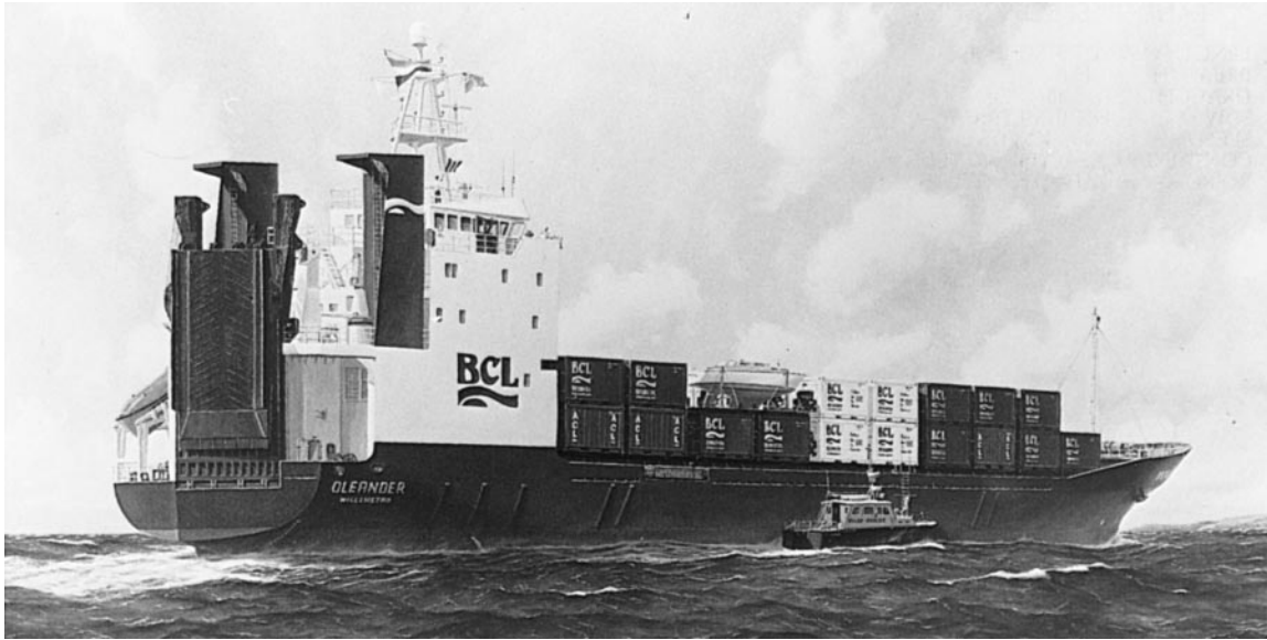
FIG. 1. Artist's view of the CMV Oleander at sea. Specifications are 118.62-m length, 19.8-m breadth, 6.26-m summer draught, 6253 metric ton deadweight, and 8.2 \text{ m s}^{-1} cruise speed. (Painting by S. J. Card, owned by Bermuda Container Lines Ltd.)
